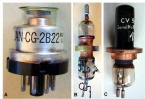
Fig. 7.2.2 - Vacuum diodes used as TR switches. A) <u>2B22</u> was a General Electric lighthouse UHF diode, also used as TR switch. B) GEC E1248 coaxial diode, approved as <u>CV8</u>, was designed in 1940 to operate as switch in a coaxial line. No known use in operational equipment. C) Marconi DS103, approved as <u>CV94</u>, was used in Type 960 high power radar, switching 450 kW peak pulses at 90 MHz. (Click on the image to enlarge)
