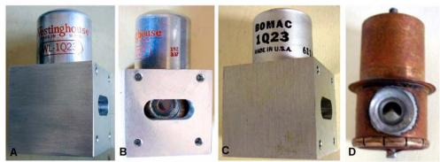
Fig. 7.2.5 - Reference cavities. <u>1023</u> resonates at 9280 MHz with unloaded Q around 2000. Here three photos of cavities complete with waveguide mount and (D) the photo of the copper resonator. (Click on the image to enlarge)
